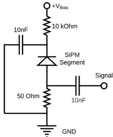
Figure 8: A simplified SiPM readout circuit diagram [9].
